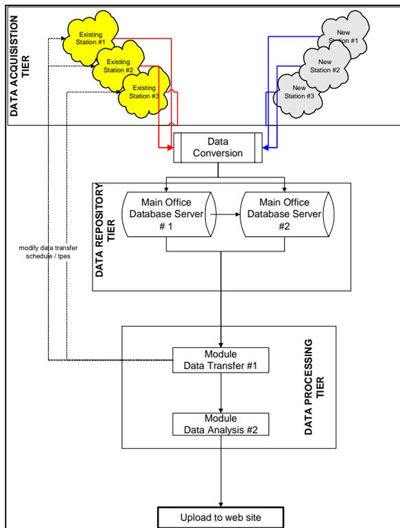
Figure 1. System design flow chart
