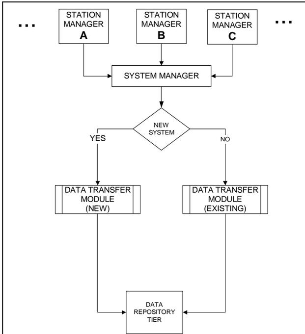
Figure 3. Data processing design flow chart
