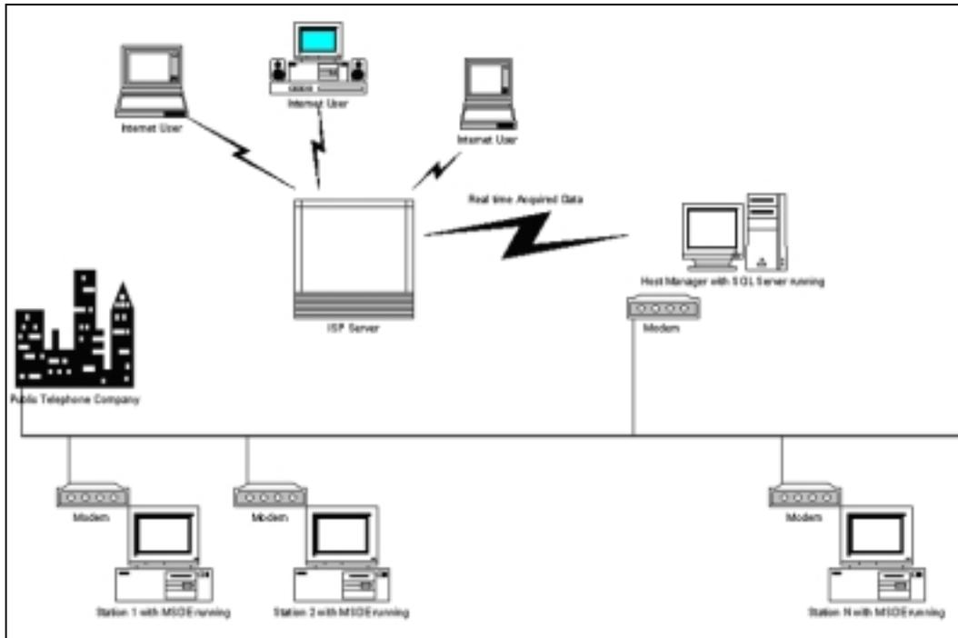
Figure 4. Air Quality Monitoring System Structure.
