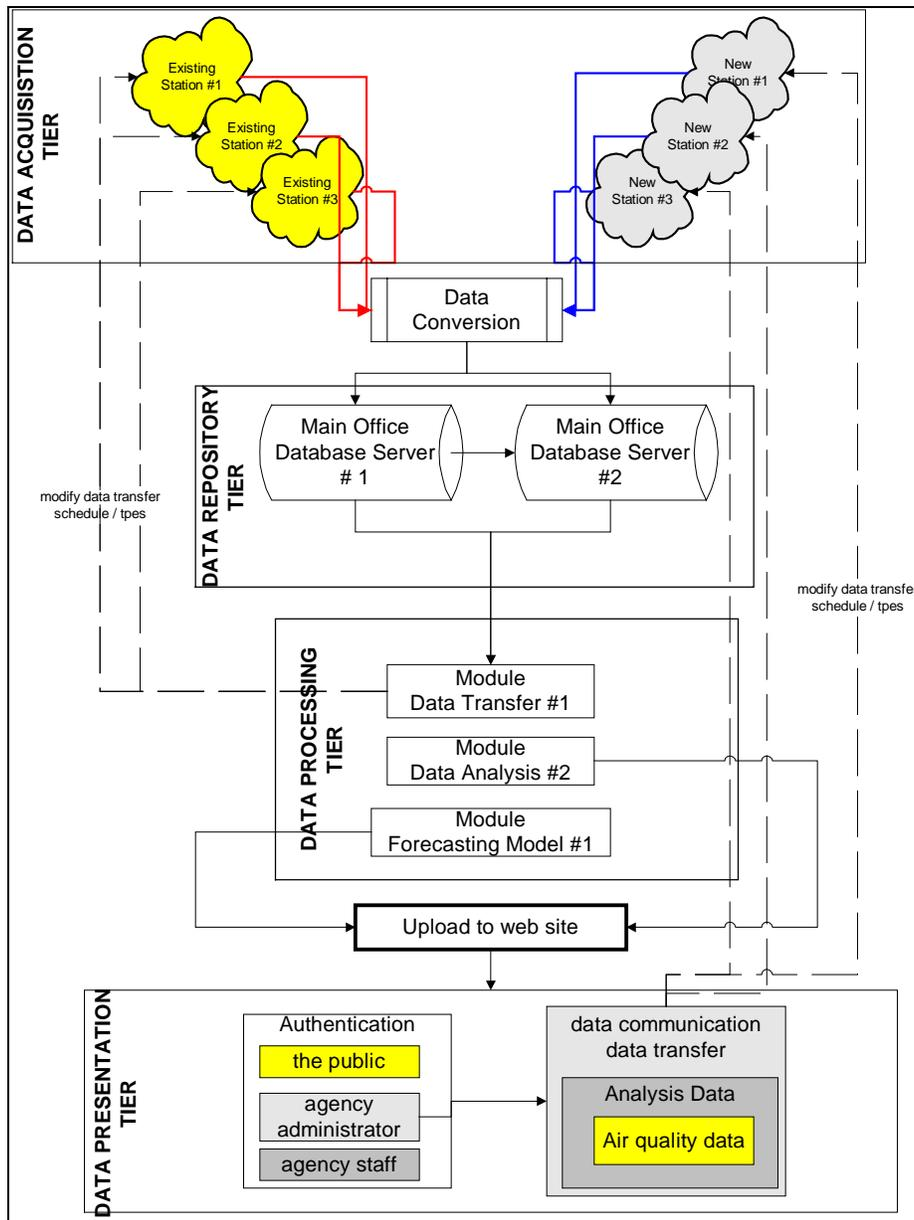
Figure 1. System design flow chart
