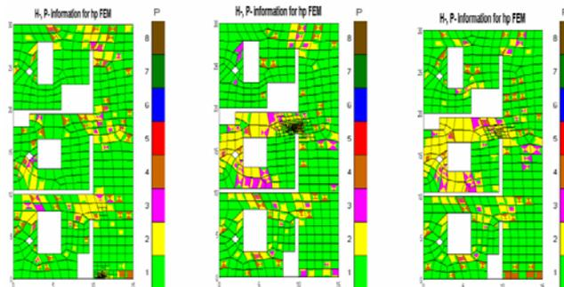
Figure 4 Final hp-adaptive FEM meshes for three cases
