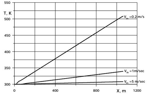
Figure 5. The drift wall temperature distribution along the drift for several values of the velocity of the air at the inlet (the number of canisters is 67, the thermal loading is  $345.2 \text{ W/m}^2$ )
