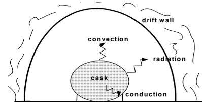
Figure 1. Modes of heat transfer associated with the cask and drift interior.
