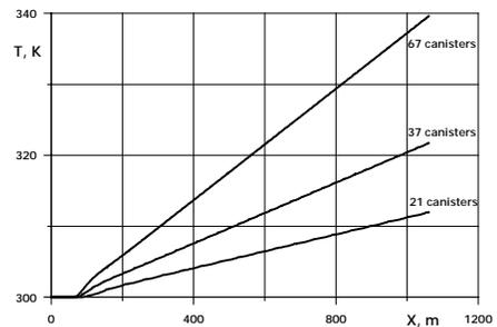
Figure 6. The drift wall temperature distribution along the drift for several numbers of canisters (the thermal loading is  $345.2 \text{ W/m}^2$ , the velocity of the air at the inlet is  $1 \text{ m/sec}$ )
