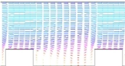
Figure 10. Velocity vectors in the middle of the drift (the number of canisters is 67, the thermal loading is  $345.2 \text{ W/m}^2$ , the velocity of the air at the inlet is  $1 \text{ m/sec}$ )
