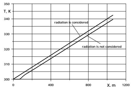
Figure 7. The drift wall temperature distribution along the drift when the radiation heat transfer is considered and not considered (the number of canisters is 67, the thermal loading is  $345.2 \text{ W/m}^2$ , the velocity of the air at the inlet is  $1 \text{ m/sec}$ )
