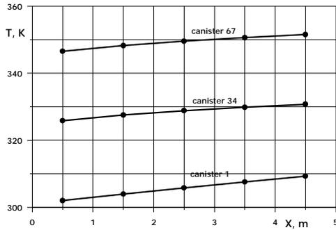
Figure 8. Distribution of the temperature on the surfaces of canisters 1, 34, 67 along the canister's relative length (the number of canisters is 67, the thermal loading is  $345.2 \text{ W/m}^2$ , the velocity of the air at the inlet is  $1 \text{ m/sec}$ )
