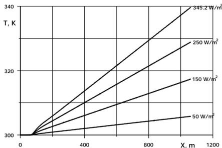
Figure 4. The drift wall temperature distribution along the drift for several thermal loadings (the number of canisters is 67, the velocity of the air at the inlet is  $1 \text{ m/sec}$ )
