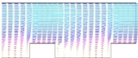
Figure 11. Velocity vectors at the end of the drift (the number of canisters is 67, the thermal loading is  $345.2 \text{ W/m}^2$ , the velocity of the air at the inlet is  $1 \text{ m/sec}$ )
